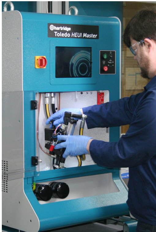
Installing an injector
