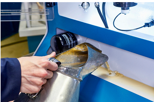
You must use ISO3114 calibration fluid
