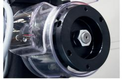
The coupling guard & safety interlocks ensure maximum possible protection for HK1400 users
