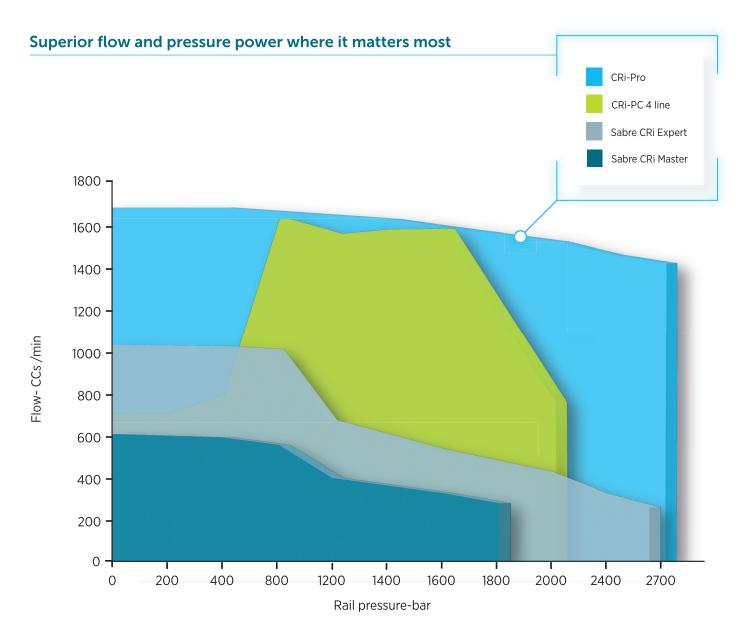
The CRi-Pro hydraulic operating envelope shows the CRi-Pro delivering optimum hydraulic performance at all levels of flow and rail pressure to cater to even the most demanding injectors.
